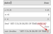
Although eval() does not display its result, you can view the resulting Hub command string after executing the command by inspecting any of the following special variables.
